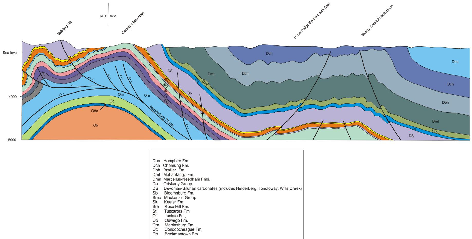
Figure 3. Northwest-to-southeast Structure cross section of Morgan County across strike, from near Flintstone, MD to Jones Creek, WV. From Dean et al. (1995). No vertical exaggeration.
